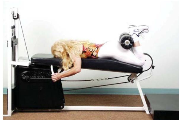
**The Vintage Nautilus Prone Leg Curl. This machine is re-engineered by Ken Hutchins to provide maximum resistance decrease at full knee flexion. To accomplish this, part of the frame has been cut away to provide a pass for the drive belt. Please read the text on page 1 to visualize the performance issues encountered with this device.**
